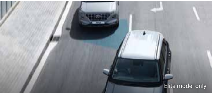
Blind-Spot Collision Warning (BCW) 2 When driving at a speed of 30km/h or higher, the BCW function will alert the driver to vehicles that enter or are in the blind spot, to help avoid potential collisions during lane changes.
