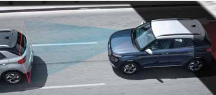
Forward Collision-Avoidance Assist (FCA) Using camera data, the FCA system autonomously activates the brakes when it detects dangerous and sudden braking by the car ahead, or movement of pedestrians on the road.
