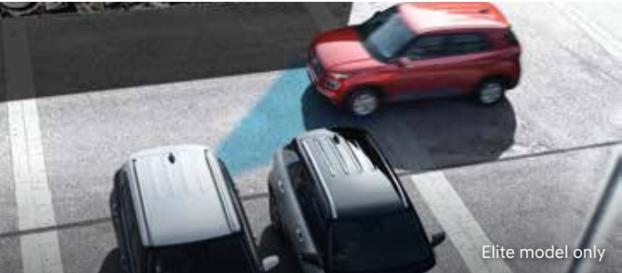
Rear Cross-Traffic Collision Warning 2 (RCCW) RCCW monitors for traffic approaching on either side of the Venue when reversing out of perpendicular parking spaces. Should RCCW detect a vehicle approaching, an audible warning will sound, with a visual warning displayed on the dash cluster.
