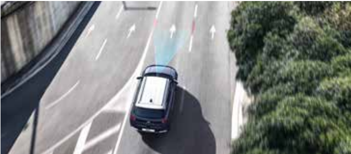
Lane Keeping Assist (LKA) LKA provides steering intervention to assist the Venue in staying between lane markings. When the Venue strays from the intended lane without indicators being activated, the LKA system will send out an audible sound and a visual warning within the cluster.
