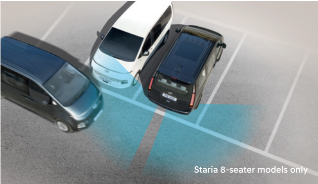
Rear Cross-Traffic Collision-Avoidance Assist (RCCA) RCCA warns of the approach of a vehicle across the rearward path when reversing and, if necessary, emergency braking is applied.
