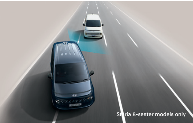
Blind-Spot Collision-Avoidance Assist (BCA) When operating the turn signal switch to change lanes, if there is a risk of collision with a rear side vehicle, the system provides a warning. After the warning, if the risk of collision increases, the function automatically controls the vehicle to help avoid a collision. If exiting a parallel parking spot and there is a risk of collision with a rear side vehicle, the function automatically assists with emergency braking.
