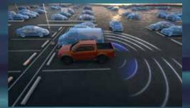
REVERSING CAMERA WITH REAR CROSS TRAFFIC ALERT (RCTA): Monitors your surrounding area while reversing warnings should an object approach from the left or right.
