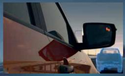
BLIND SPOT MONITOR (BSM): Provides a visual warning in your side mirrors when an obstacle is approaching in your blind spot.
