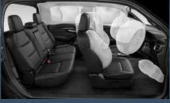
EIGHT AIRBAGS: For ultimate protection, every D-Max comes with eight airbags including a centre airbag to protect front seat occupants in side-on collisions.
