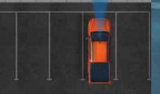
MISACCELERATION MITIGATION: In slow moving areas such as car parks, the stereo cameras determine whether the accelerator has been applied accidentally. Should a potential collision be detected. the brakes are automatically applied. (Automatic Transmission only).
