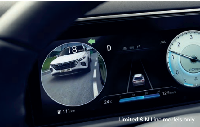
Blind-Spot View Monitor (BVM) When the turn signals are activated, the rear-side image of the corresponding direction is displayed in the cluster.
